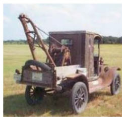
Truck w/chain hoist [14]
